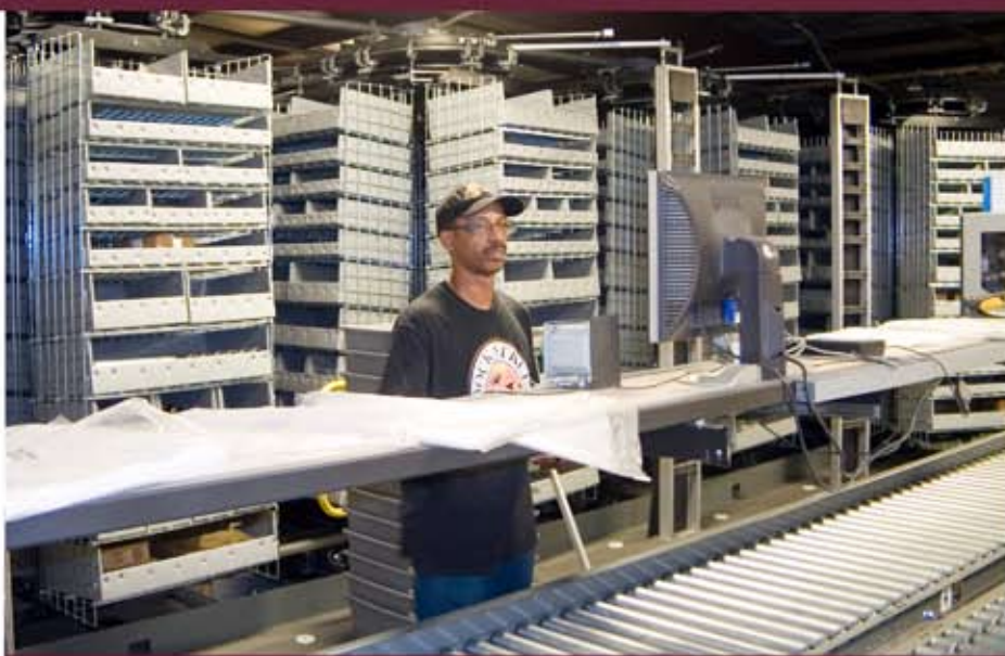
The carousel system consists of 10 carousels and manages an inventory of 60,000 SKUs.
