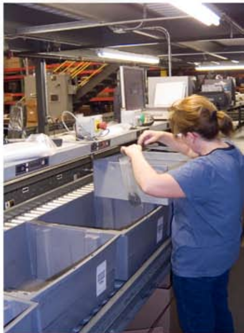
Totes are automatically delivered to operators, who are directed by pick- and put-to-light technologies.
