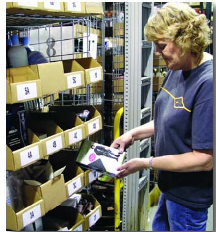
Items are brought to the operator and batch picked increasing throughput and eliminating 10 miles of walking per day.
